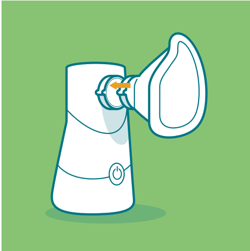
Mouthpiece attachment to the nebulizer is guided by shape coding and confirmed via perceptible tactile and audible feedback.
