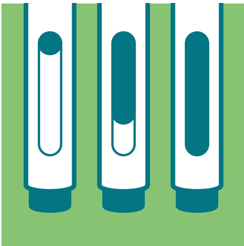
An auto-injector viewing window turning yellow after administering the medication will show the user that all medication has been delivered and the device cannot be used again.
